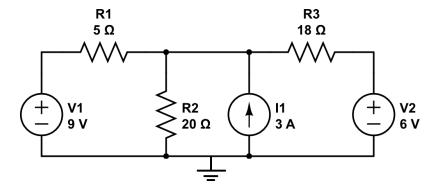
8. Draw the Thevenin equivalent circuit with R3 as the load resistor. (4)
