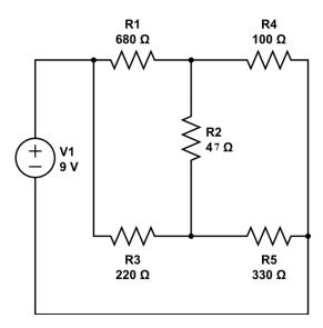
3. Calculate the equivalent resistance of the entire circuit (3)
