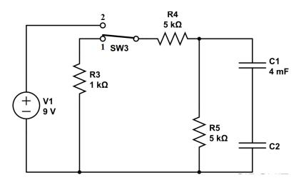
12. After a very long period of time, the switch is moved from position 1 to position 2 and then after 2 time constants, the voltage across capacitor 1 is .972748 V. What is the time constant? (5)
