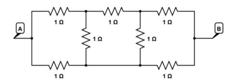
Find the equivalent resistance between points A and B. \_\_\_\_\_\_ What would the equivalent capacitance be if all the resistors were replaced with 1 Farad capacitors? \_\_\_\_\_\_
