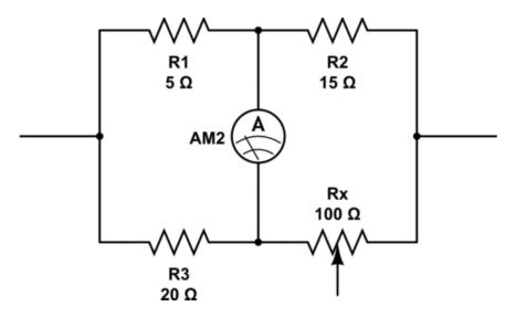
3. What value of R<sub>x</sub> allows for greatest power dissipation of said resistor?
