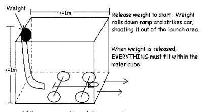
All the energy used to push the car must come from a falling mass of <=1 kg.
