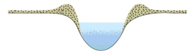
18. Consider a river with a width of 7 m, depth of 2m, and a mean velocity of 45 cm/s.
