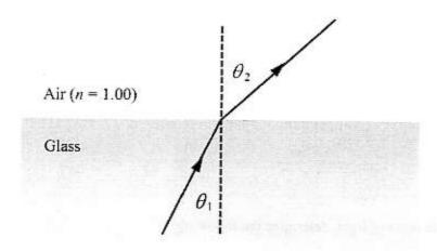
In an experiment, a beam of monochromatic light (wavelength  $\lambda = 675$  nm in air) passes from glass into air, as shown above. The incident and refracted angles are  $\theta_1$  and  $\theta_2$ , respectively. In the experiment, angle  $\theta_2$  is measured for varying angles of incidence  $\theta_1$ , and the sines of these measured angles are used to obtain the line shown in the following graph.
