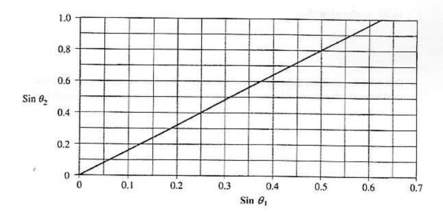
a. Assuming an index of refraction of 1.00 for air, use the graph to determine a value for the index of refraction n<sub>g</sub> of the glass for this color light. Explain how you obtained this value, making clear what information was obtained from the graph, and how it was used.
