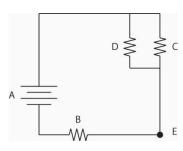
18. Consider the circuit shown above. In what direction (from the battery) is electron (e) flow going in the circuit, and in what direction is conventional current going?
